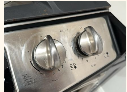
The knobs on the cooktop are worn and unreadable.
